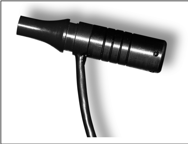
Diagram 2: Ultrasound probe (Aviso, Quantel Medical, Clermont Ferrand, France) with integrated laser fixation device.
